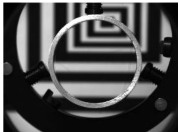
Fig. 5: Perspective error due to common optics (left image) and perspective error absence (right image) with a telecentric lens.
